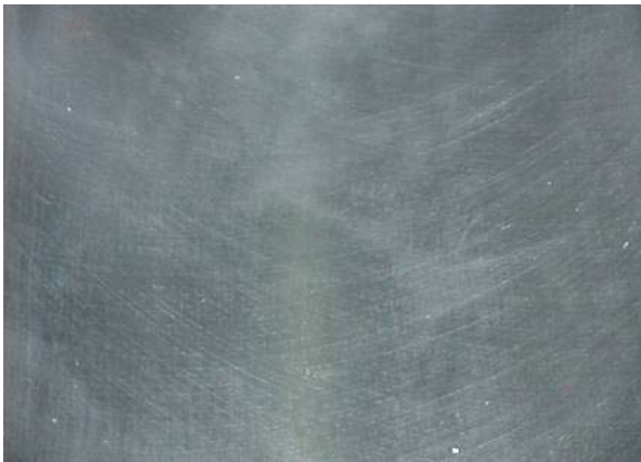
Figure 6-19. Phosphate-Coated Cylinder w/ Revised Hone Pattern
