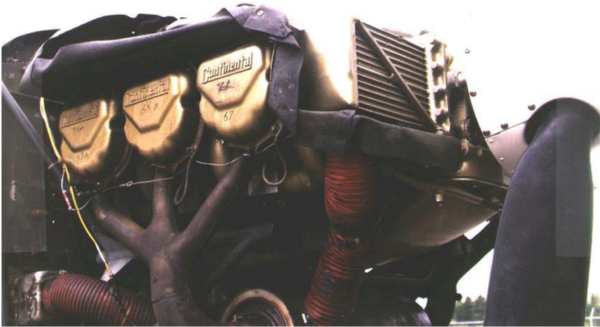
Figure 6-25. Improperly Positioned Baffle Seals
