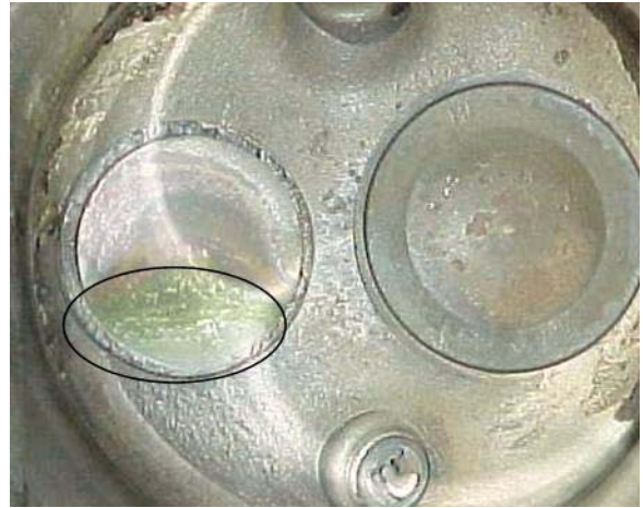
Figure 6-18. Burned Exhaust Valve
