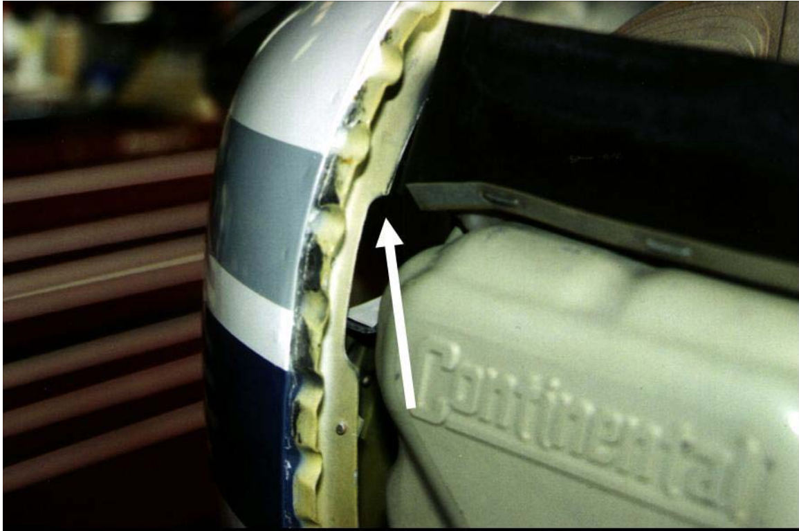
Figure 6-29. Cooling Loss Due to Gaps in Baffle Seals
