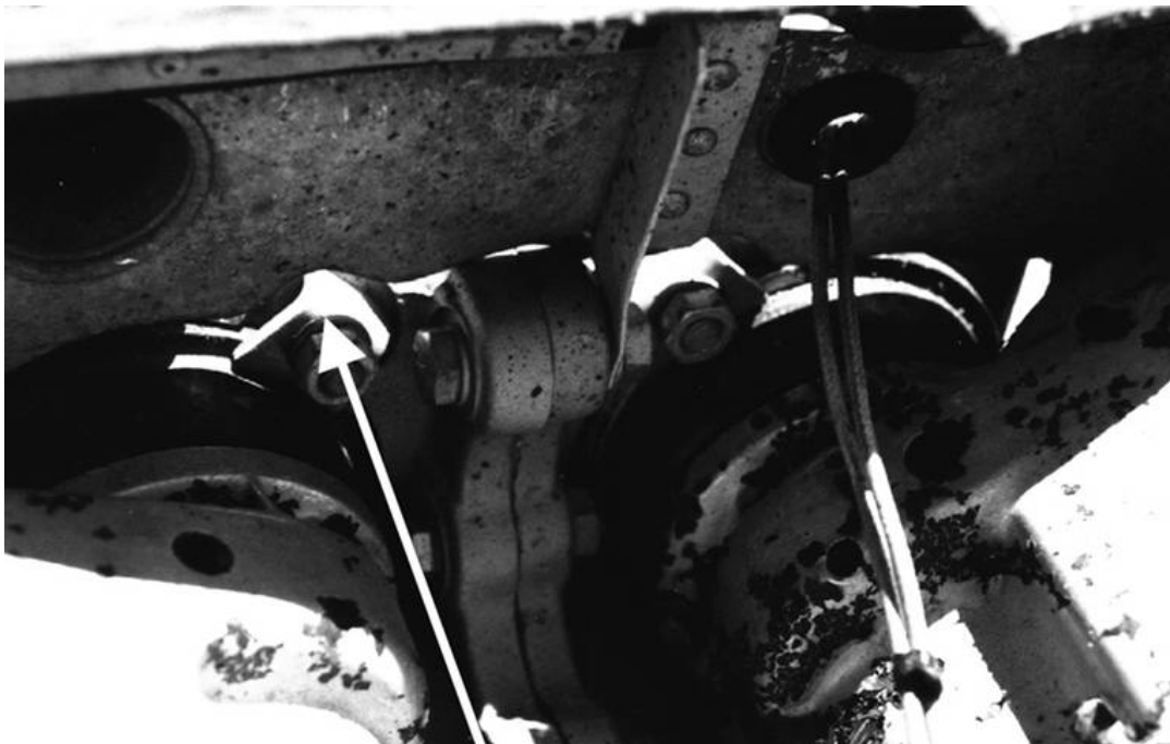
Figure 6-28. Aft and Side Baffles with Air Gaps
