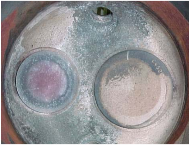
Figure 6-17. Normal Combustion Chamber
