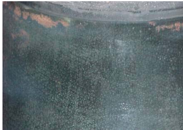
Figure 6-20. Phosphated Cylinder Bore
