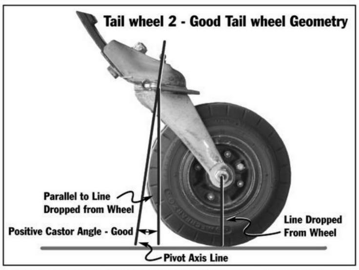
Tail wheel with positive and negative castor angles—exaggerated.
