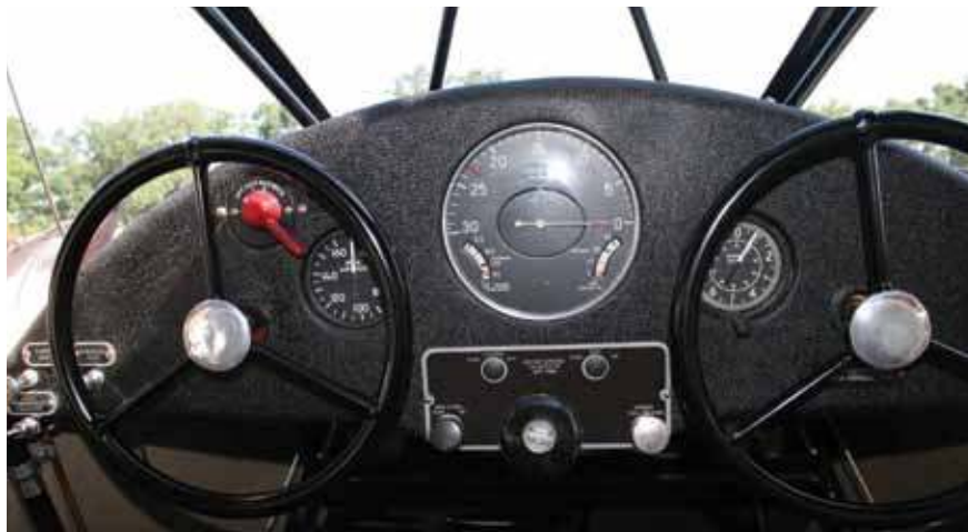
The instrument panel is dominated by the large tachometer/engine instrument combination in the center.
