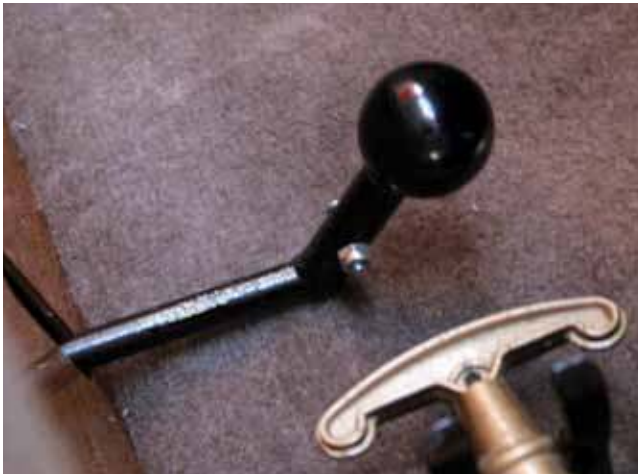
The black handle is for the wobble pump, and the brass handle is for the fire extinguisher.
