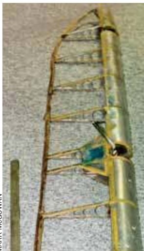
The aileron, with the fabric removed.
