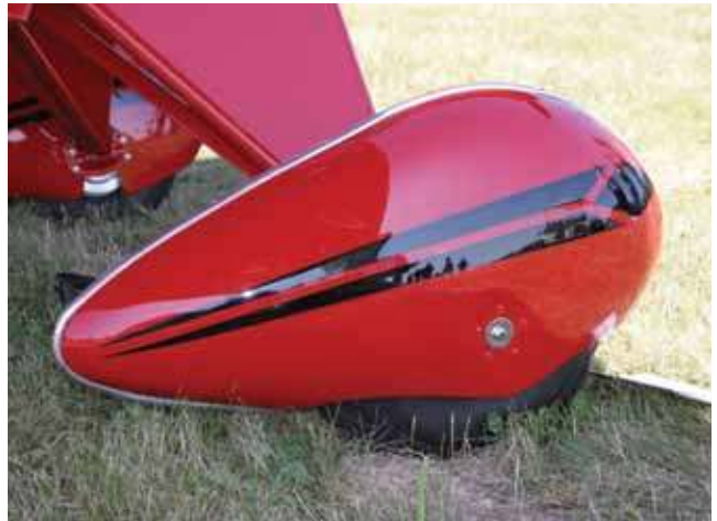
The prewar wheel pants feature a center-seam trim crafted out of aluminum.
