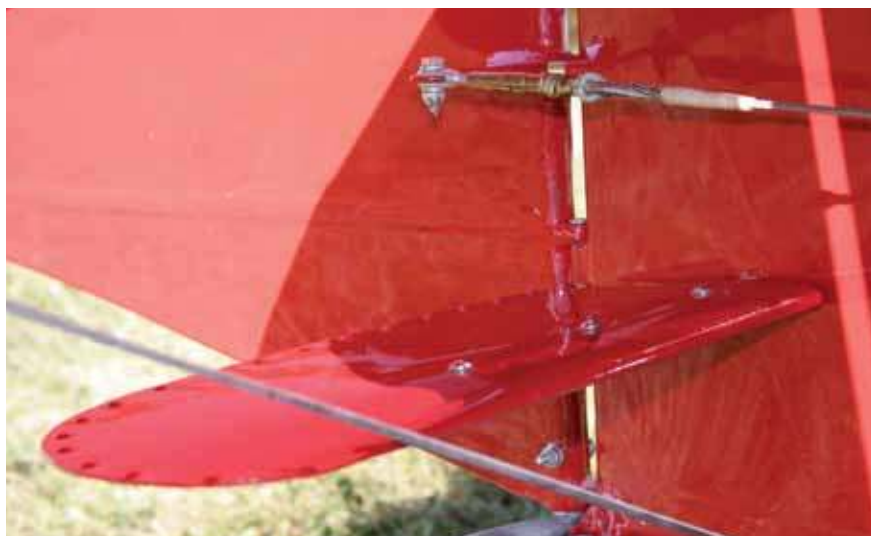
Close-up view of one of the two Flettner trim tabs that are mounted on the fuselage beneath the horizontal stabilizer.
