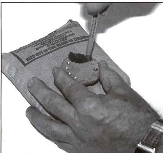
Using the pencil and Scotchbrite pad, apply pressure and rotate in each of the brass indents to clean any impurities and corrosion.
