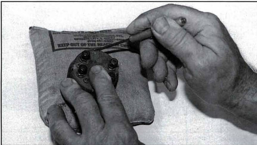
Using a small flat blade pocket screwdriver, carefully open each of the four retaining tabs holding the fiber backplate.
