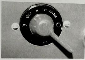
The standard looking AAF Type A7 with the nice large knob that has a handle. While the exterior portion of these switches is nearly bulletproof, the interior components are subject to wear and will eventually be unserviceable.
