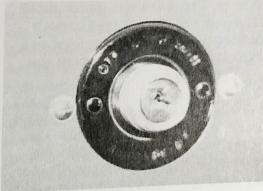
With the knob removed, the modern key magneto switch is seen.
