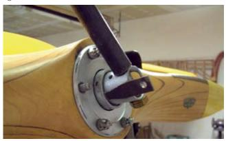
The snap ring retention tool has been inserted into the snap ring opening, and the pipe extension is in place. The prop hub nut is now ready to be rotated counterclockwise approximately two to two-and-a-half turns.
