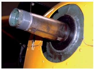
The exposed tapered crankshaft should be inspected for corrosion, then thoroughly cleaned and lightly lubricated for prop installation.
