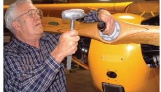
While applying light pressure to the back side of the prop, insert the steel shaft into the hub nut and tap lightly with either a rubber mallet or lead hammer. The light pressure prevents the crankshaft journals from banging against the engine case when applying the light tapping to the inserted steel shaft.
