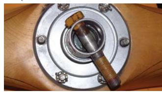
A 5/8-inch by 4-inch Grade 8 bolt is inserted through the prop hub locking nut. Note that the spinner-mounting bracket has been removed for complete access to the hub.
