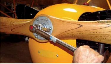
The special socket is in place, and correct torque values are now applied to the hub nut.
