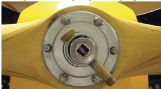
The specially designed hub socket has been inserted into the hub locking nut and the Grade 8 bolt inserted through the nut and socket. This setup allows for properly torquing the hub nut using a torque wrench.
