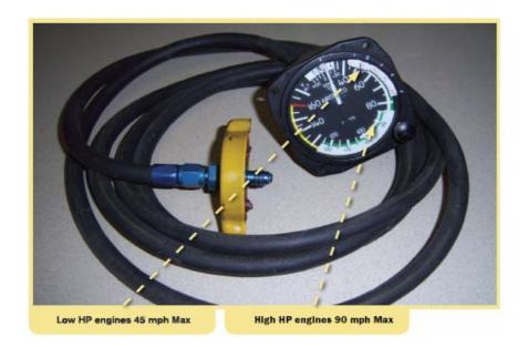
If you see higher gauge readings you should inspect your engine breather system for restrictions. Also make sure the breather outlet is not being restricted by cowl flaps, the cowling, or being located in a high air pressure area. The best outlet location, to start with, is at the bottom edge of the firewall then adjust as needed from there.
