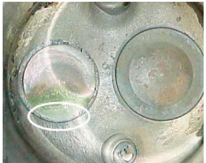
Burned exhaust valve. Note edge of valve face that has lost all combustion residue and striations moving toward center of valve.
