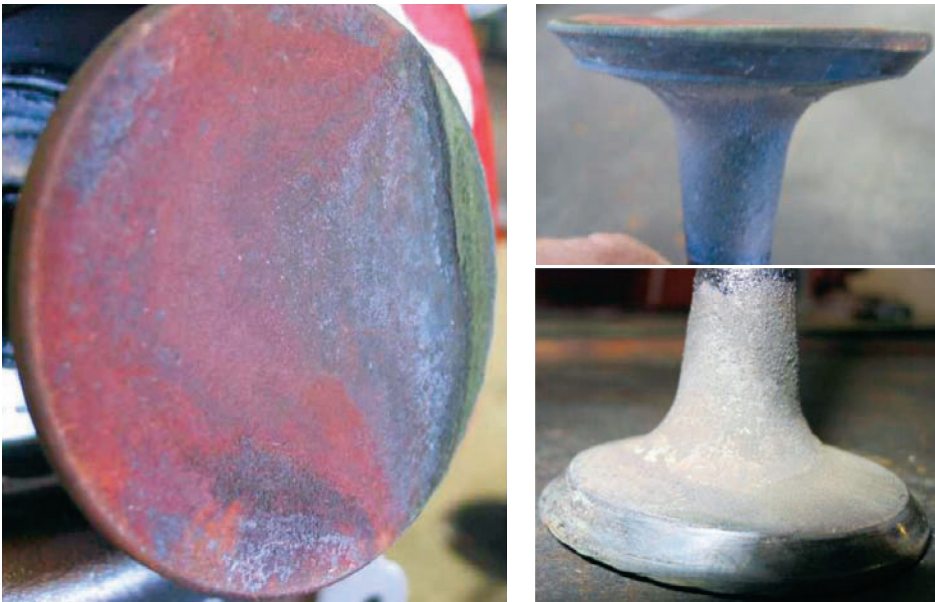
FIGURE 4: Borecope inspection of this TCM exhaust valve revealed the characteristic signature of a burned valve - an asymmetrical pattern of deposits with an area nearly devoid of deposits where the valve is overheating (left). Side views of the removed valve (right) show just how warped and eroded it had become. A few more hours in service would almost certainly have resulted in complete loss of power in the cylinder.
