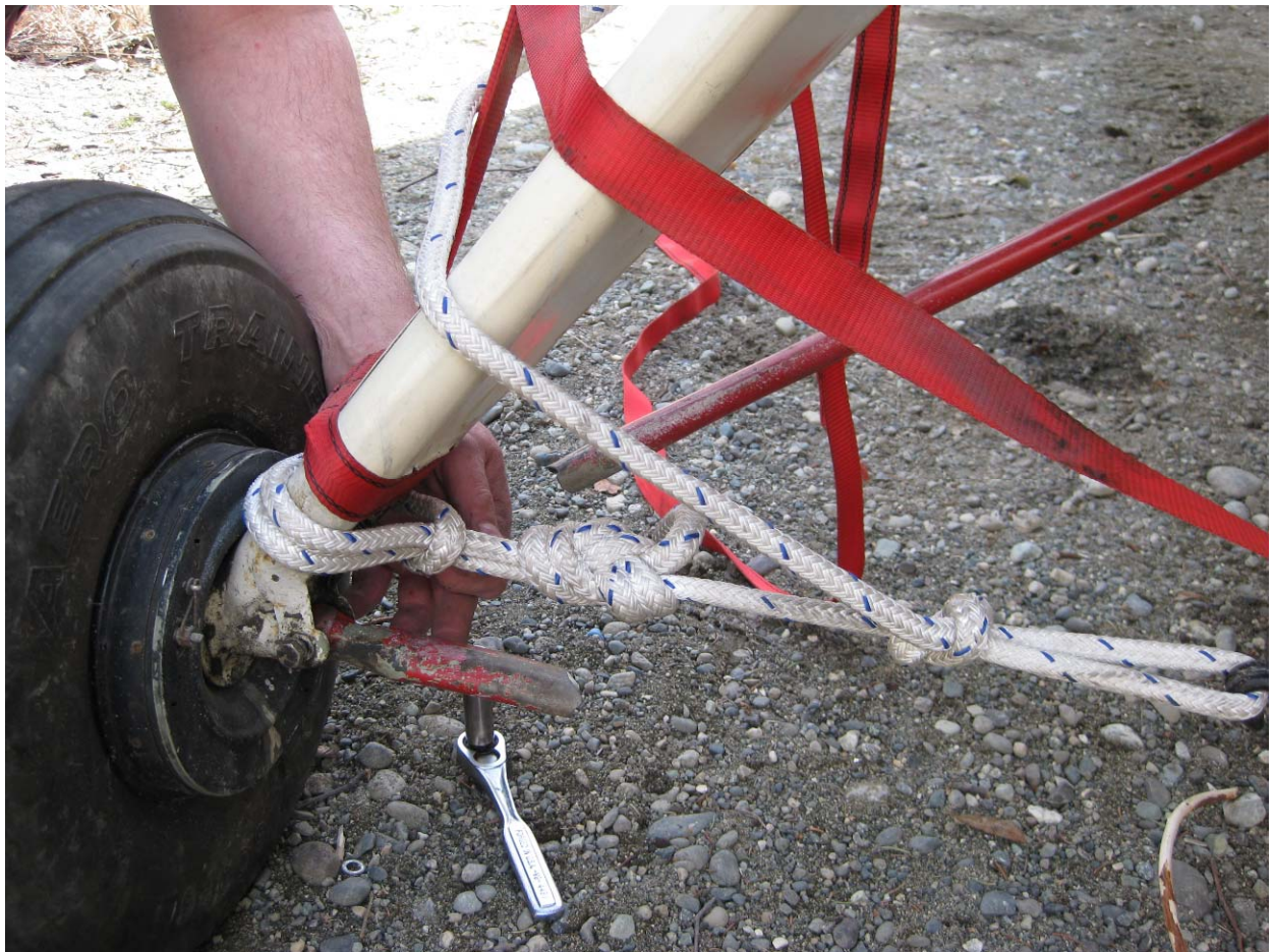
Failed Tie Strut on RH Main Gear
