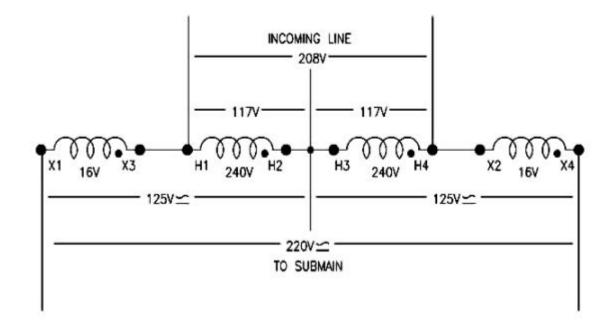
Easy, huh? We simply made use of the ratio rather than the voltage ratings. There is a price to pay, though. The current rating in amps will be the same whether we excite it with 240 or 480. So, we must use the higher rating to calculate the current rating.
