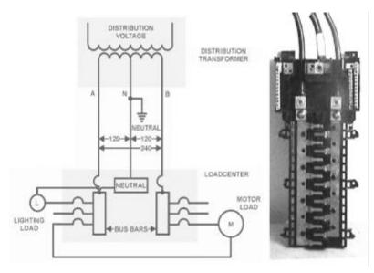
So, let's look a little closer at this ground business. The main load center for the house has either lugs at the top of busbars or а large breaker that spans the width of the box. If the large breaker is there, it is the "Main Disconnect" for the service. No breaker? Then the meter is the disconnect.
