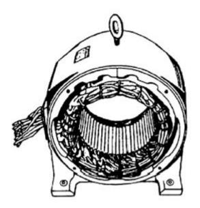
The net result is an electromagnet that literally rotates inside the frame of the motor. The speed of this rotating field is called the "Synchronous Speed". Many times I have connected a motor without the "guts' and spun a steel ball inside the stator frame to illustrate this field. The ball is actually pulled to the center of the frame as it spins.
