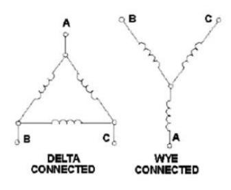
There are two ways to make up poly-phase transformers. **Star**, or **Wye**, has the three windings tied to a common point, and to a phase. **Delta** is connected phase to phase.
