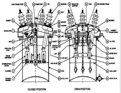
Oil break switches are usually spring operated in both conditions. Then motors rewind the springs, "charging" them for the next operation. The reasoning here is that the faster the contact closes or opens, the less damage from melting off tiny pieces of copper.
