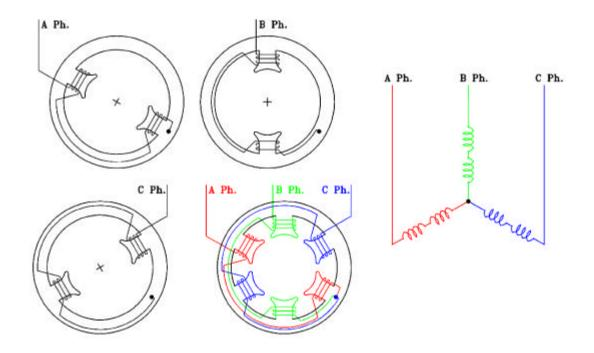
As the alternator produces three sine waves from a rotating magnet, we now are looking at reproducing that magnet inside the motor. Essentially reversing the process. You will note that the times shown in the illustration are indicative of the position of the rotating magnet in the alternator.
