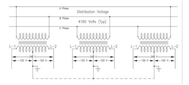
The dashed line on the bottom does not exist as a specific conductor. Through bonding and the natural conductivity of the ground, there is a low impedence path between neutrals from the various transformers. The bars in each transformer indicate "magnetic isolation".
