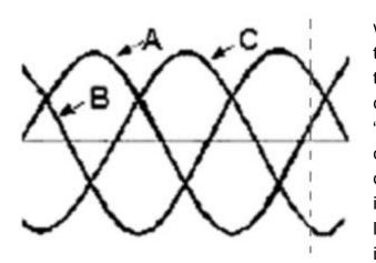
The 1.73 is a multiplier we will encounter everywhere in three phase systems. Remember this wave form from the conversation on alternators? The "X" axis, horizontal, is time. In this case, 16.6 mSec, 1/60 second, one cycle. The "Y" axis, vertical, is current as it is delivered to the load. Look to the right side, there is a dotted line indicating a time
