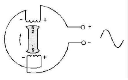
The output waveform *is* a bit misleading. Notice that the north pole is at maximum flux density relative to the upper coil. Thus, at this instant, the output is at maximum positive. The waveform is displaying a 90 degree lag. A *minor* point, but it could be confusing. It confused me in '68.
