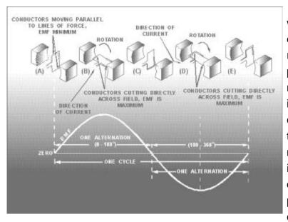
The output waveform shown is for one complete revolution of the rotor. As the conductor passes the face of the magnet, a positive current is produced. Then, as the conductor continues past the opposite face of the magnet, a negative current is produced. The strength of the magnet and its' physical relationship to the coil are what produces the
