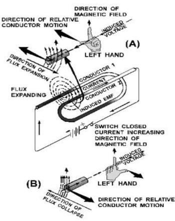
three axes, each at right angles to the others. Motion. Flux. Current. Motion is represented by the thumb. Flux by the index finger. And Current by the middle finger. The acronym MFC associated with the middle finger has gathered many crude descriptions over time. I leave them to your imagination. The association preferred by the Navy book from which I stole this picture is "My Fine Clothes" This association is suitable for mixed and company is easy to remember.
