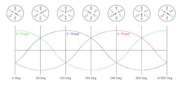
At time "0" Phase B has maximum current sinking to positive and creating a magnetic south as indicated by the arrow head. At time "120", the south pole has moved to align with the Phase C coil. Then again at time "240", the south pole has moved to align with Phase A. You will note that as each phase swings negative, current is sourcing through the second half of each coil. As at time "60, 180, and 300".
