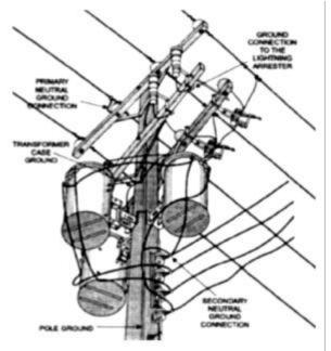
Very small three phase drops simply have the transformers mounted on a service pole. Such an installation is similar to a residential single phase service, just with the additional transformers.
