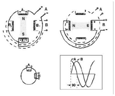
phase by 90 degrees. Such an alternator is shown here.
