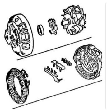
many alternators, the armature windings are brought out to insulated studs, ahead of the diodes. Most modern alternators use an internal regulator module. Such machines require extensive modification to be used for non-standard applications.
