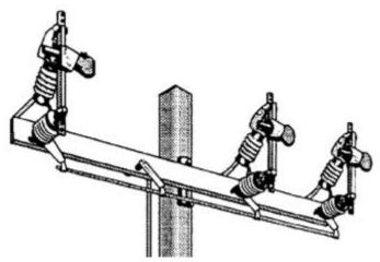
There are three types of high voltage switches. **Air break, Vacuum break**, and **Oil break**. As noted above, opening an air break switch under load is not a good thing. They are used mostly for isolation. Sure is nice to walk up and see the knife arms out and grounded before starting work. There is no question it is safe to work. They may be manually operated or motorized. Or both, as appropriate.
