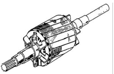
Yes, this is a conductor buried in another conductor. As will be discussed shortly, while the currents are high, voltages tend to be very small. The current will follow the path of least resistance, seldom straying outside the cage proper.
