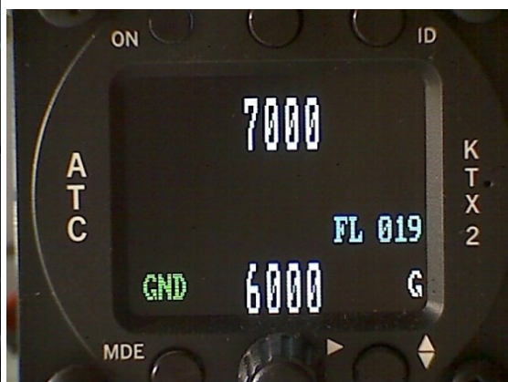
GND-switch installed, on GND
