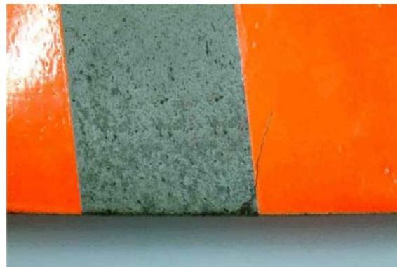
FIGURE 1-9. Blade Crack from a Nick
