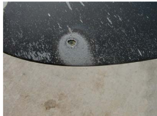
FIGURE 1-12. Lightning Strike on a Composite Surface
