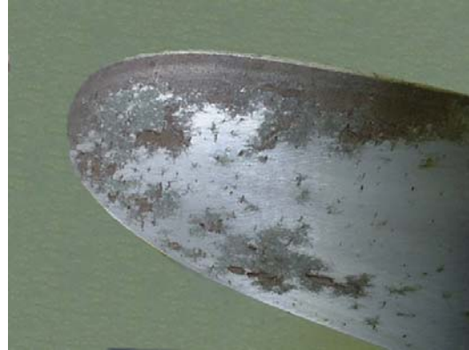
FIGURE 1-2. Polished Blade Surface Corrosion
