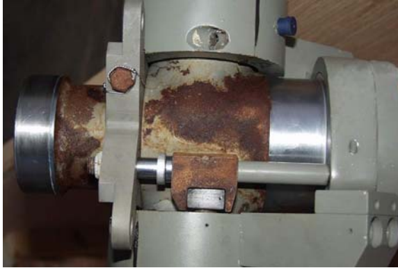
FIGURE 1-1. Hub Surface Corrosion
