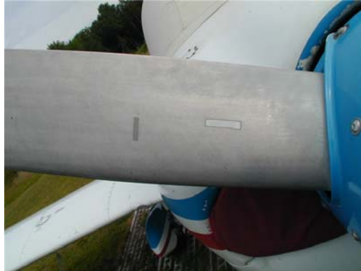
FIGURE 3-1. Balance Tape that was not Removed
