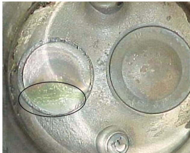
Burned Exhaust Valve
