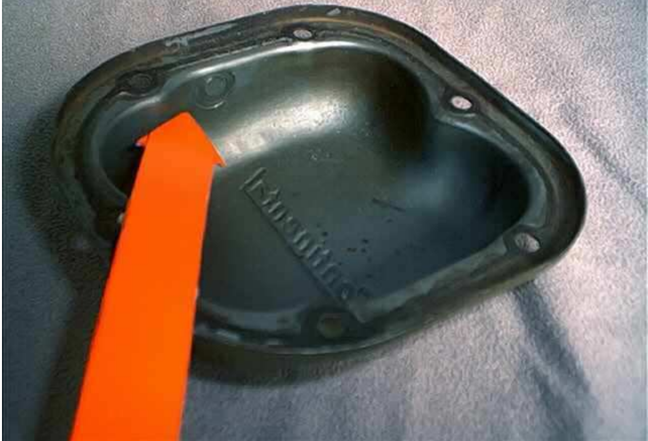
C150, O200A rocker box cover showing wear from rocker shaft
