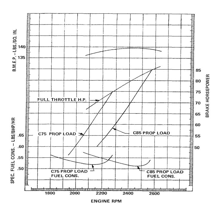
Figure 3. Model C75 & C85 - Sea Level Performance Curve
