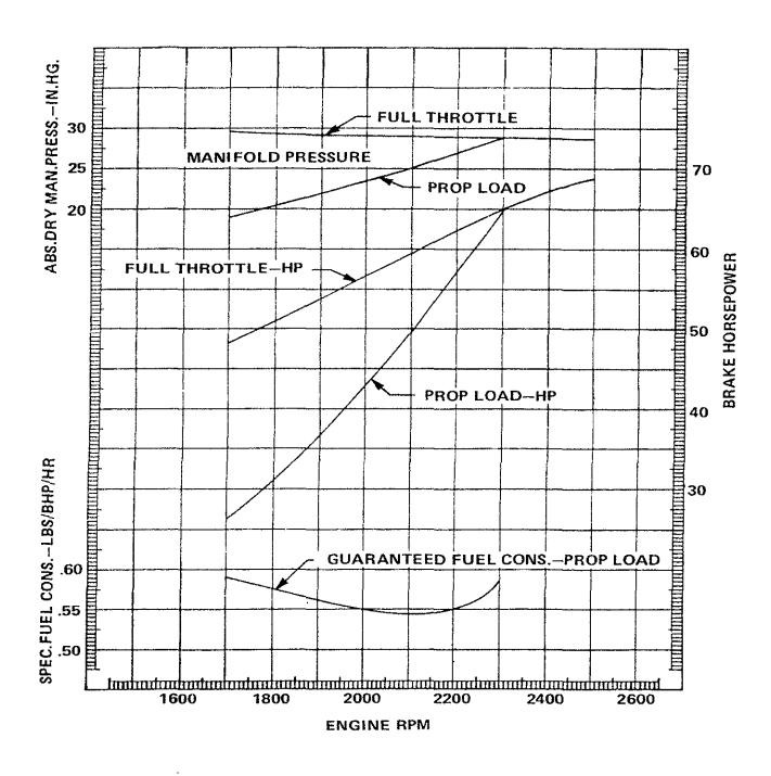
Figure 1. Model A65 - Sea Level Performance Curve
