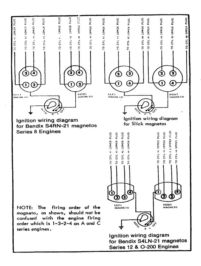
Figure 11. Ignition Wiring Diagram
