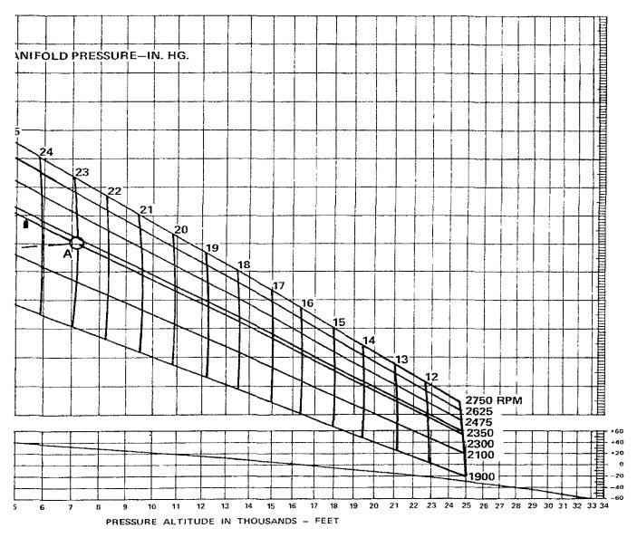
Figure 9. Model C90 — Altitude Performance Curve
