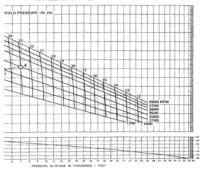
Figure 7. Model A75 — Altitude Performance Curve
