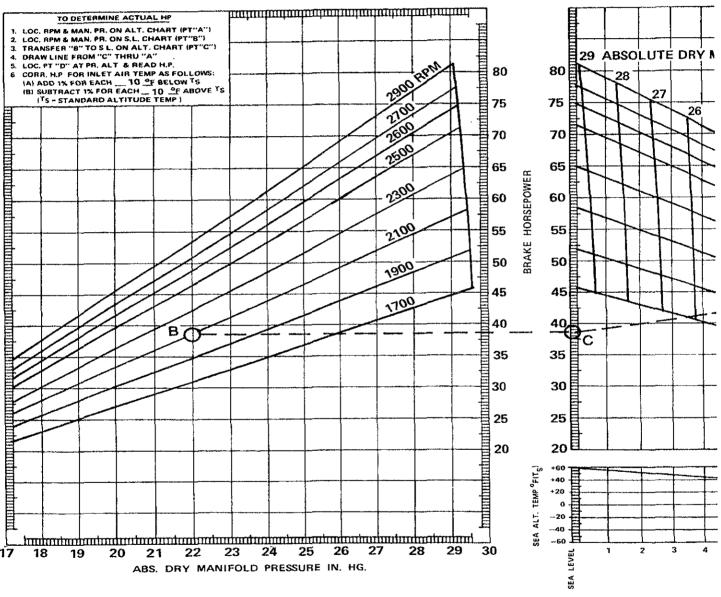
Figure 6. Model A65 - Altitude Performance Curve
