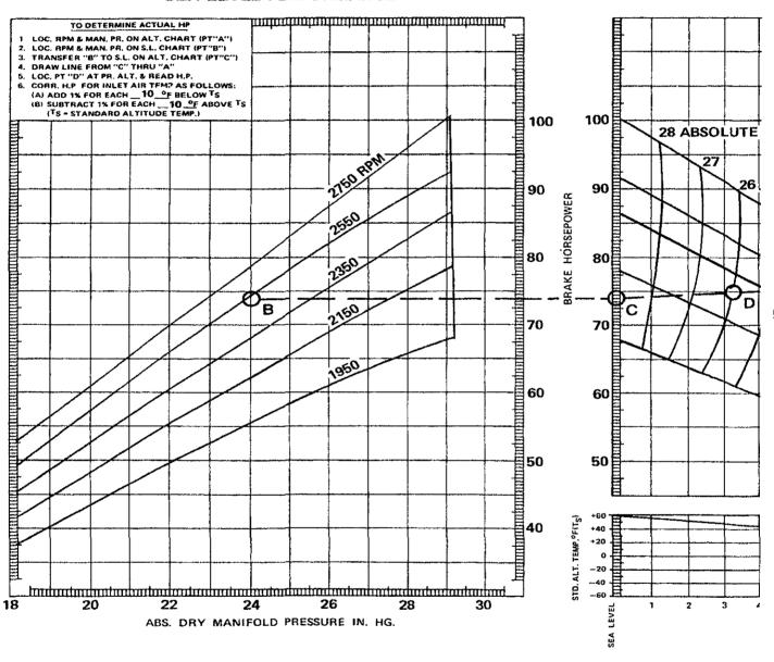
Figure 10. Model O-200 - Altitude Performance Curve
