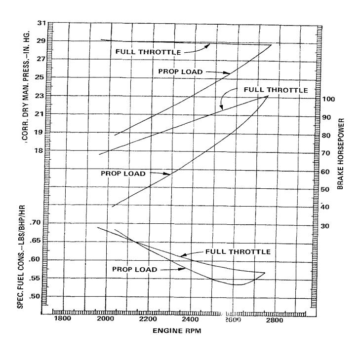
Figure 5. Model O-200 - Sea Level Performance Curve
