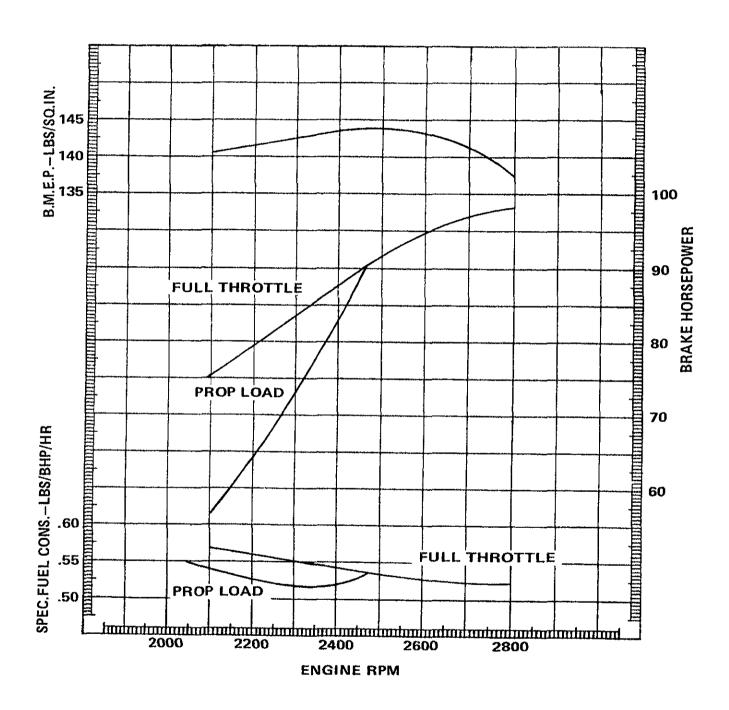
Figure 4. Model C90 - Sea Level Performance Curve
