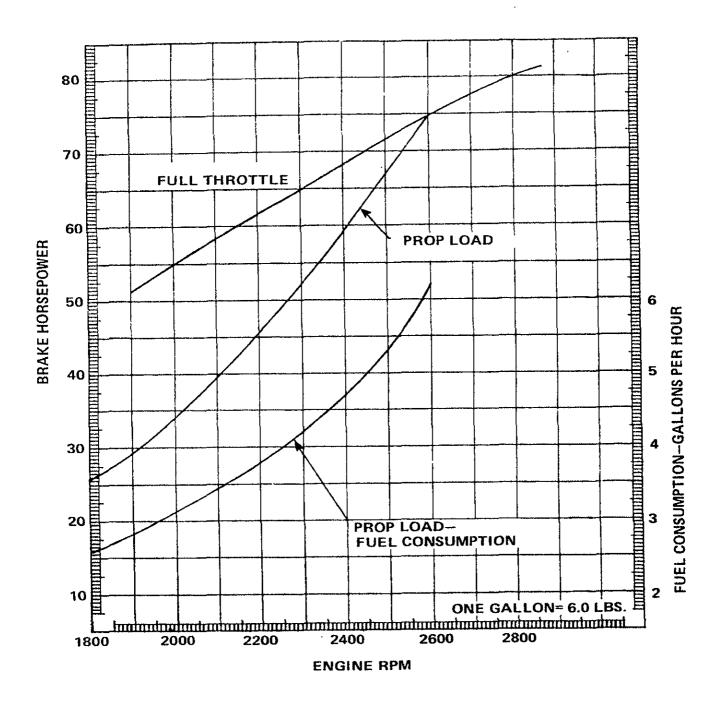
Figure 2. Model A75 – Sea Level Performance Curve
