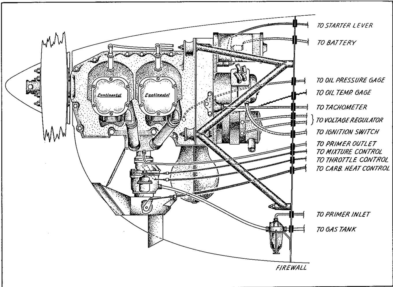
Figure 12. Typical Installation Diagram for -12, -14 & -16 Models, Side View.
