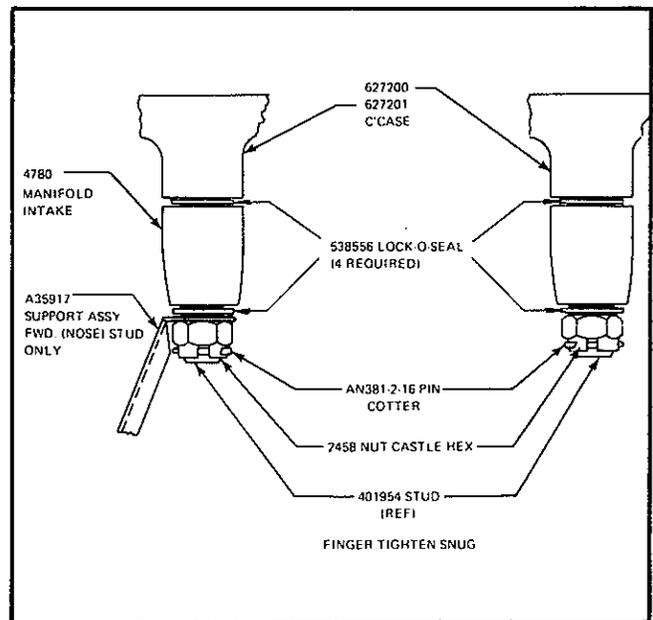
Figure 38. Install "O" Rings on Intake Manifold Studs.
