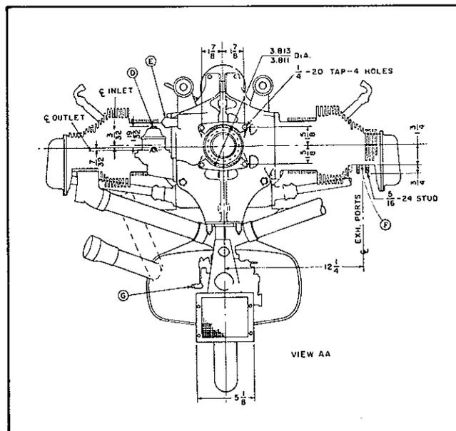
Figure 13. Installation Drawing for -12, -14 & -16 Models, Front View.
