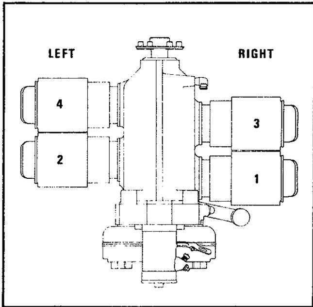
Figure 7. Cylinder Arrangement Diagram (Top View).
