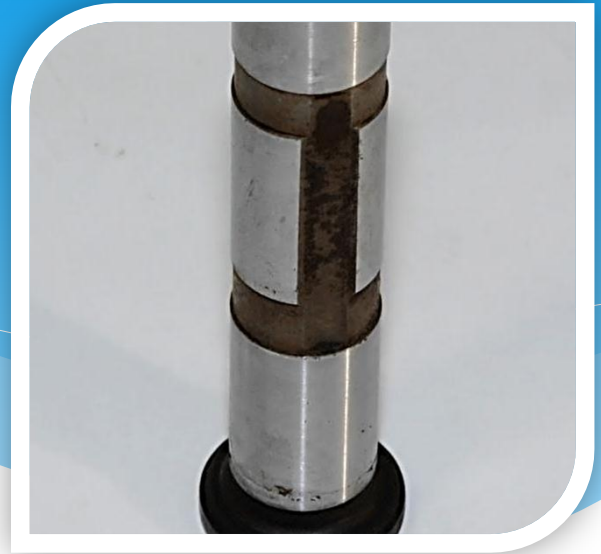
Fig. 2 Glass beads in oil transfer relief area.
