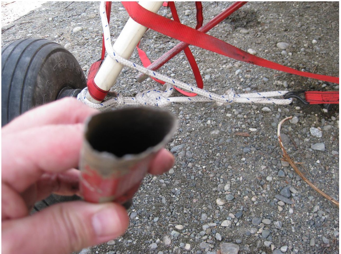
Broken End of Tie Strut (Removed from Aircraft)
