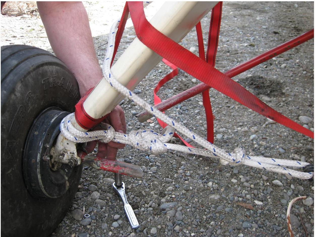
Failed Tie Strut on RH Main Gear
