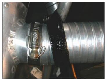
✓ So that's exactly what I did. The friction tape is coated with black gasket shellac to protect it from engine oil.
