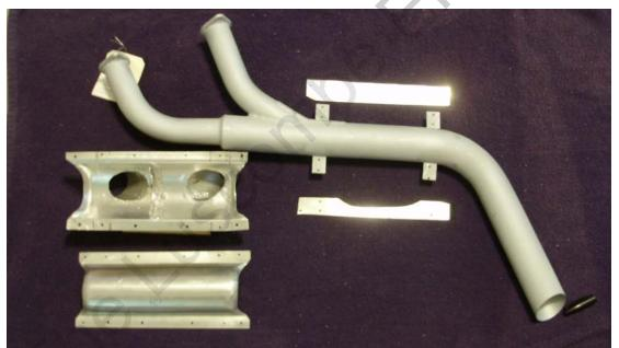
Note that the welded internal chamber baffle in the inboard muff part forces the air to flow around the outside of the exhaust stack for heating before exiting the chamber at the outlet tube:
