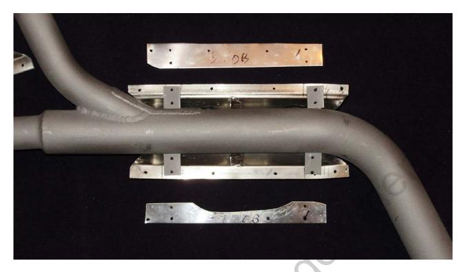
Some folks in colder climates ALSO wind small springs around the stacks to increase heat dissipation into the passing air. The baffles are used to reduce airflow speed, and to increase heat transfer into the heater airflow. Note how the baffles create a single, circuitous pathway for the air.
