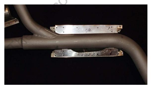
In fitting this system up, there will be some anomalies between stacks and stack manufacturers. It is usually necessary to relieve the muff where it meets the exhaust
