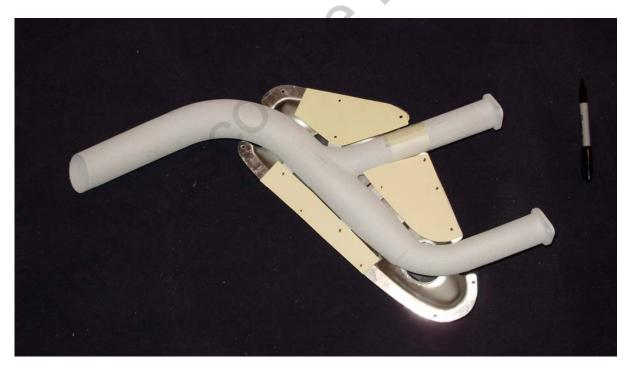
With the baffles properly mounted to the stack tabs, the clamshell muff parts are then mounted to the baffles around the perimeter flange, using screws on about a 2 to 3" center:
