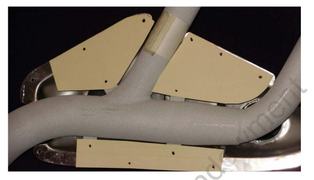
Note that the inboard carburetor heat muff clamshell has a chamber baffle that forces the air to circulate around the outside of the stacks, and to exit ONLY after a circuitous route through the muff.
