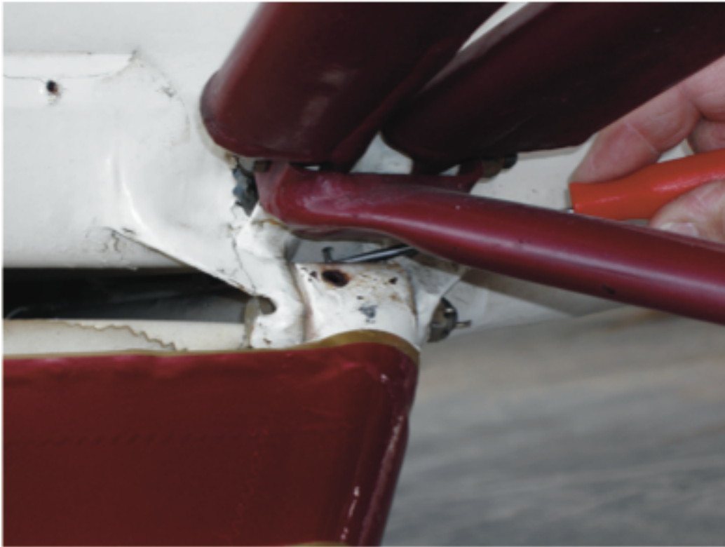
Fig. 2b Verify Drain Hole is Open
