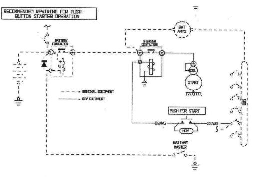
Figure 3. Push-Button Wiring
