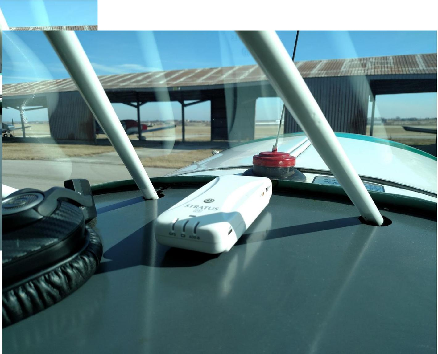
**Limit size of Velcro as it is stronger than the dash sheet metal !! Placed under heavy end of Stratus**
