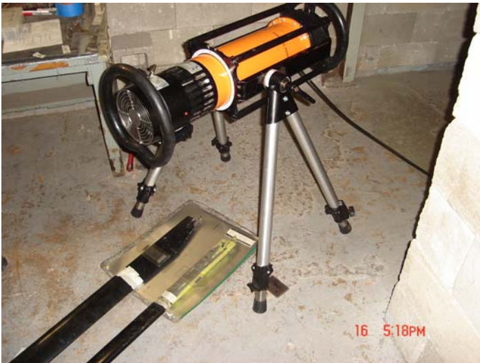
Radiographic set-up of removed struts. Struts and Cal. Std. placed on the film after removal from aircraft. .250" lead sheet placed under film to eliminate back-scatter.
