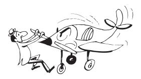
the plane. If the plane is not so equipped, certain areas of the airframe have been designated by the manufacturer as safe for push/pull pressure. Know where these points are, and just remember—for positioning, the nose is a no-no!
