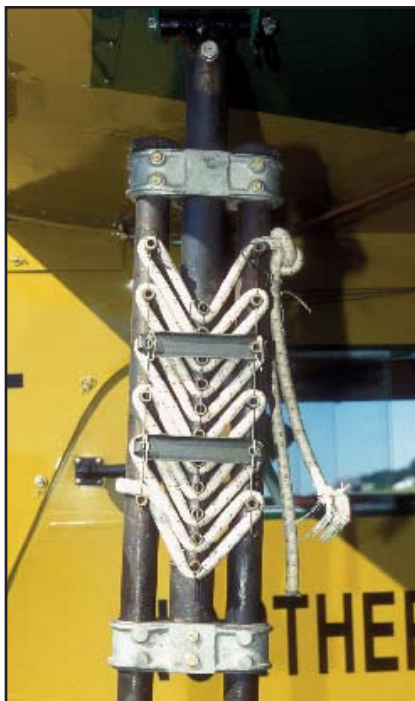
Some aircraft use multiple shock cords. This is the upper end of the landing gear of a Fokker Super Universal. A similar herringbone arrangement was used on the Ryan NYP, Spirit of St. Louis.
