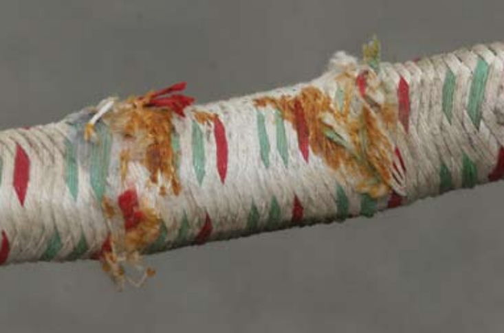
This same cord showed some signs of abrasion damage to the woven covering where the shock cord was in constant contact with the landing gear structure.
