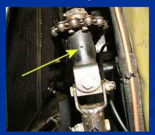
Lubricate the access hole on the bronze trim shaft
